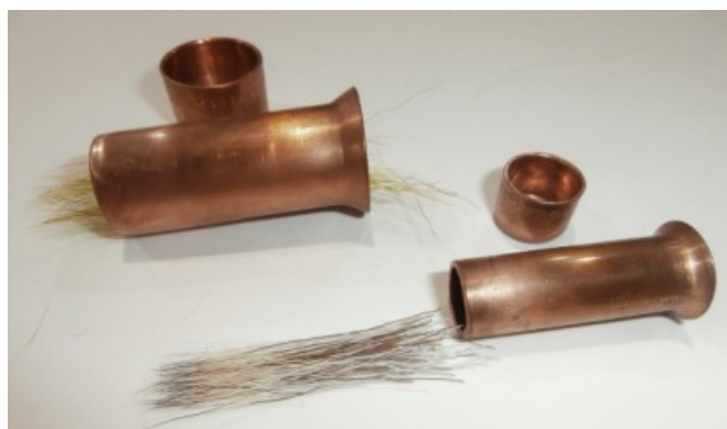
Plumbers flaring tool opens end in to the shape needed.
